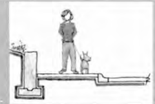
Where adjacent grades require it, or where planters or seat walls are desired, walls can be used against the sidewalk, or within the landscape.
