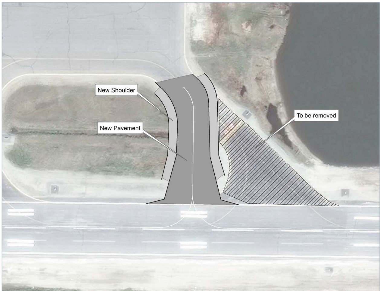
Figure 5-1 - Taxiway E Realignment
