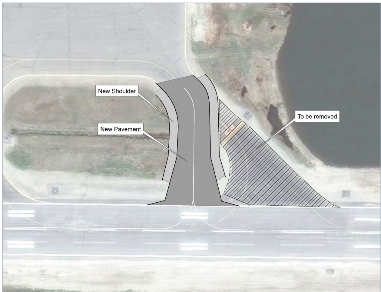
Figure 5-1 - Taxiway E Realignment
