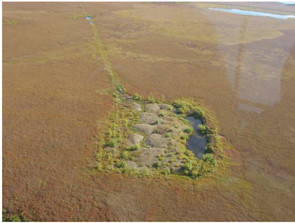
Figure 19 Former oil well drill site. Note the thermal degradation of the pad and access road.
