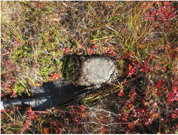
Figure 5 Wet saturated silt just below the surface at the potential ridge site, frozen ground at less than 18 inch depth.
