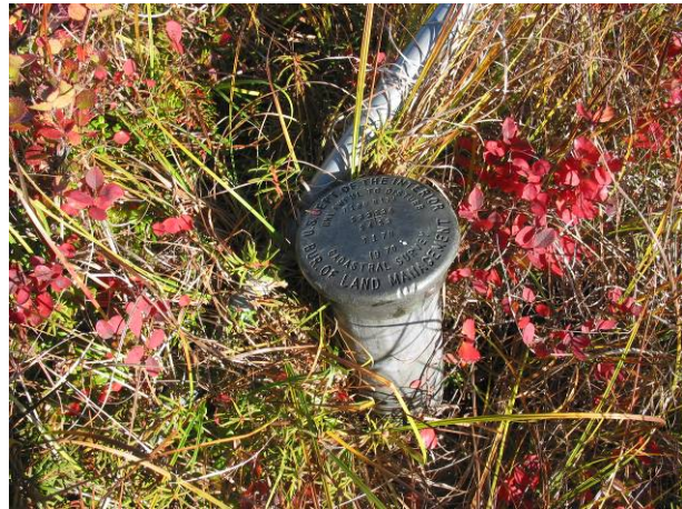
Figure 4 Section corner monument was found near the potential ridge site (S33,34 T18N R17W and S4, 3 T17N)
