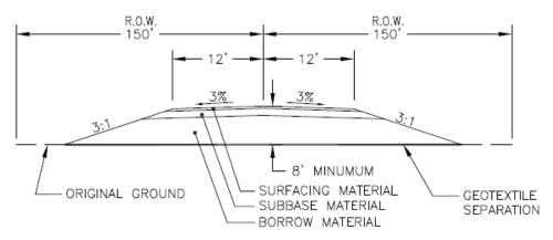
Figure 9 - Recommended Typical Section
