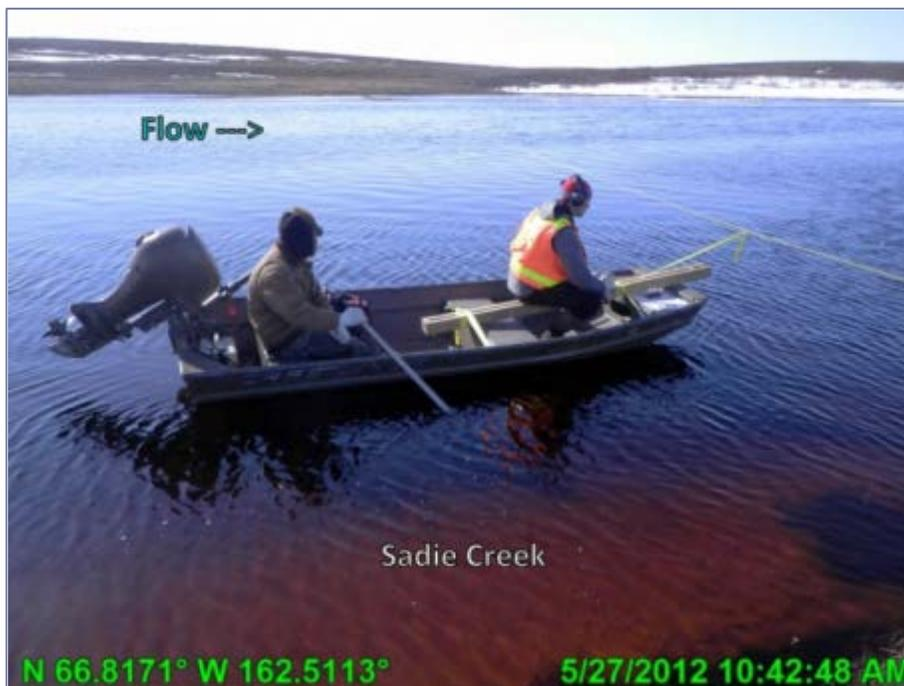
PHOTO 3.3: DIRECT-DISCHARGE MEASUREMENT AT SC1, LOOKING SOUTHEAST; MAY 27, 2012
