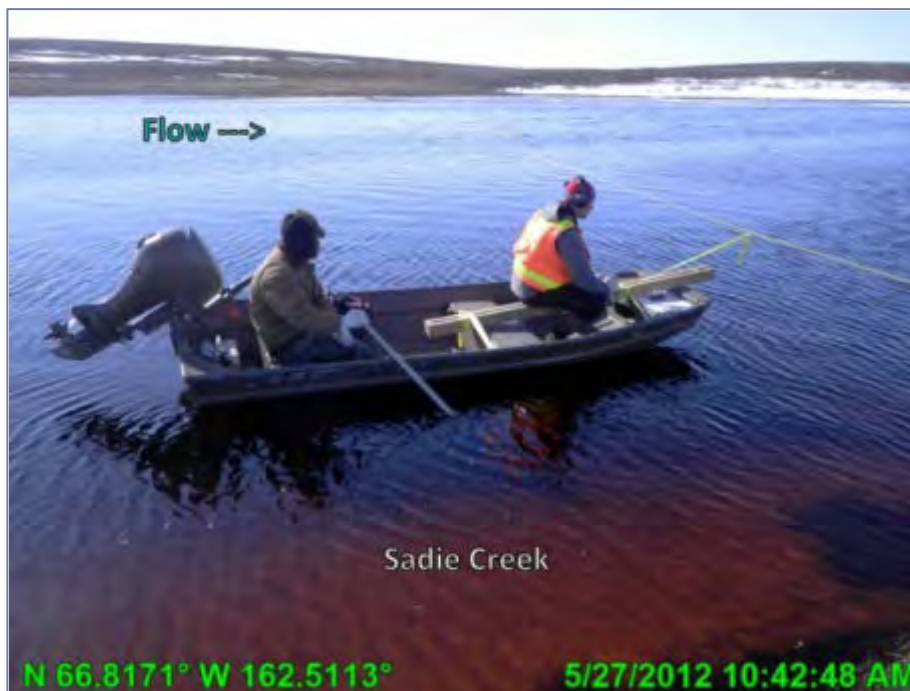
PHOTO 3.3: DIRECT-DISCHARGE MEASUREMENT AT SC1, LOOKING SOUTHEAST; MAY 27, 2012
