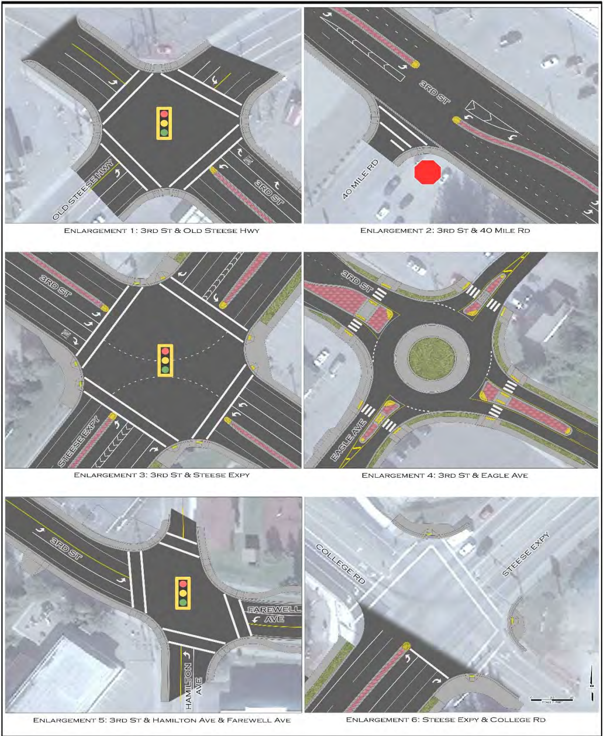
3RD STREET WIDENING ENLARGEMENT PLAN VIEWS
