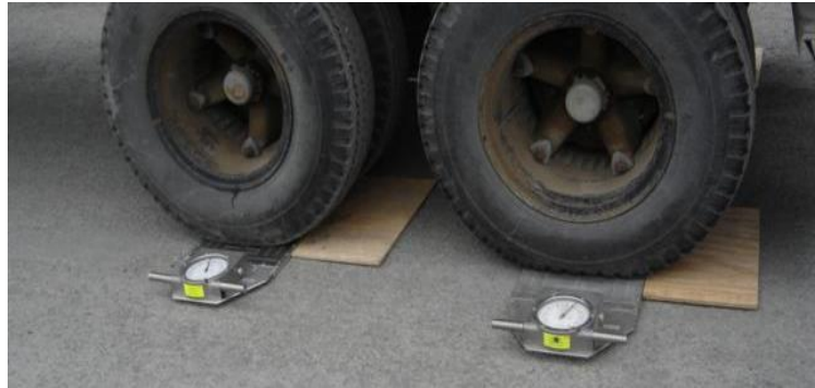
Haenni scales weighing a double axle.
