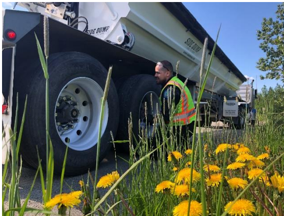
A Commercial Vehicle Compliance Inspector performing a Level I and checking wheel fasteners on a CMV.
