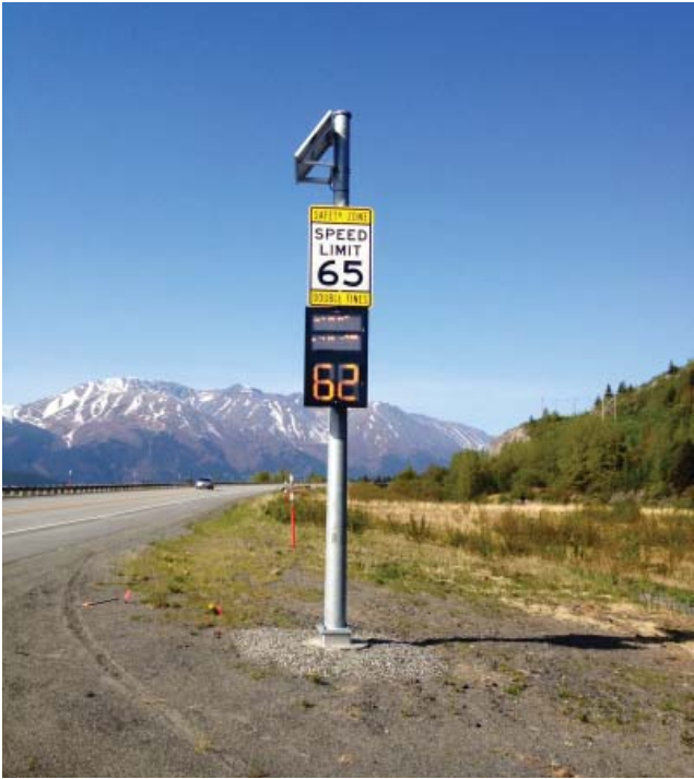
Intelligent Speed Limit Sign indicating speed of approaching vehicles is 62 MPH
