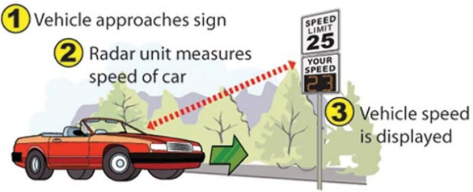
Diagram of how feedback signs work courtesy of http://www.wsbeng.com/services/driver-feedback-signs
