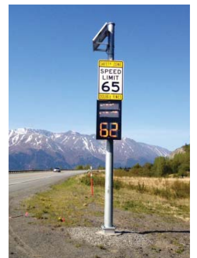
Intelligent Speed Limit Sign indicating speed of approaching vehicles is 62 MPH
