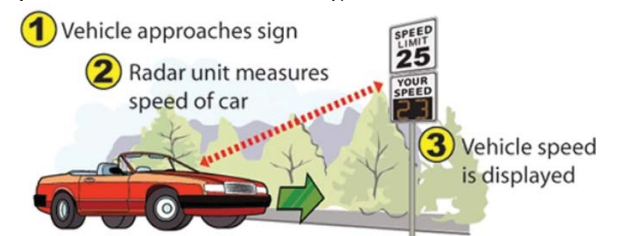
Diagram of how feedback signs work courtesy of http://www.wsbeng.com/services/driver-feedback-signs
