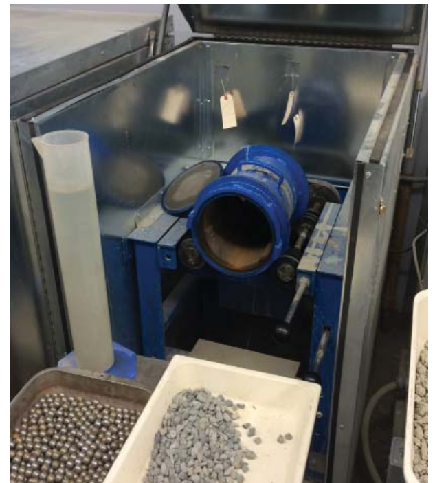
The “Nordic Abrasion Test” is used to determine how well the aggregate will stand up to studded tire wear.
