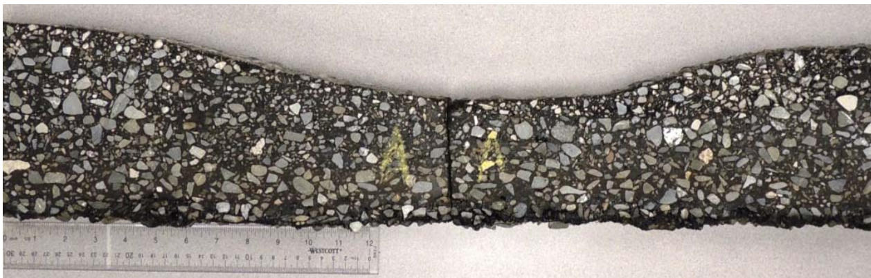
This cross section of rutted pavement was cut from a steep section of Eagle River Loop Road and illustrates the impact of studded tire use in high traffic areas throughout Central Region.
