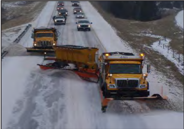
The tow plow has been used successfully in Missouri since 2005 but, this winter will see its first use in Alaska.
