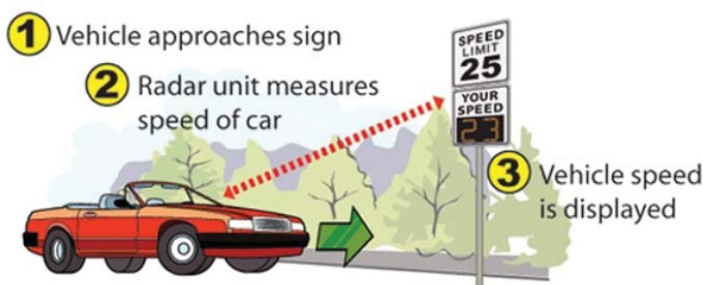
Diagram of how feedback signs work courtesy of http://www.wsbg.com/services/driver-feedback-signs
