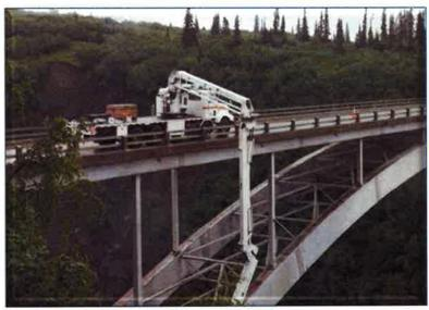
Bridge Truck currently in the process to be replaced. The boom can no longer be certified for safe use.
